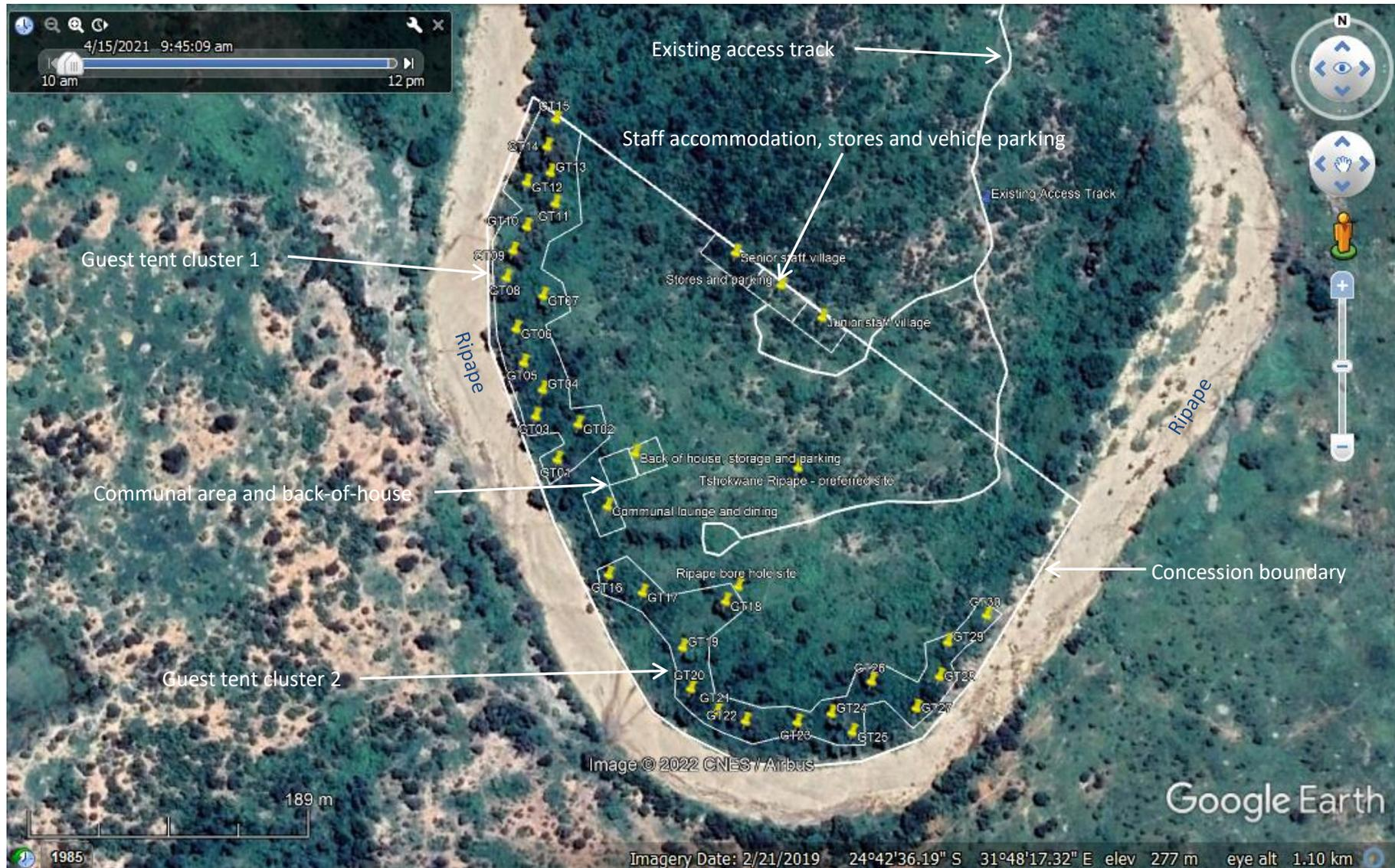
Figure 6: The detailed layout of the Tshokwane Ripape camp on the preferred site. To be viewed in conjunction with Figure 4.
