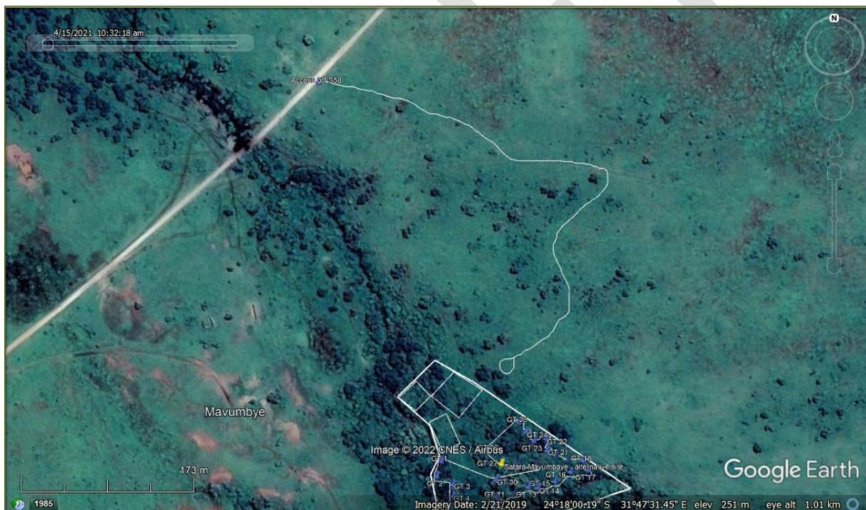
**Figure 13:** The position of the access track that will need to be constructed for access to the Satara Mavumbye alternative site.
